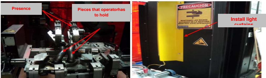
Figure 3. Robotic Cell 1 Fixture 1 Manifold with Changes Required
