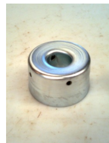
Figure 3. Original hand tool made of galvanized sheet metal
