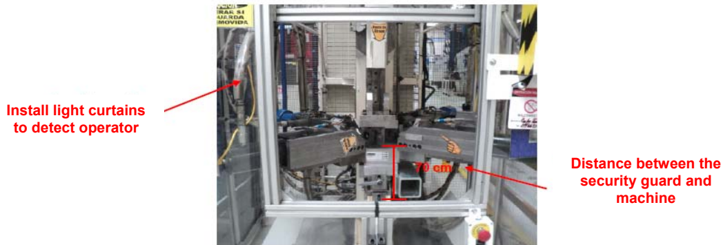
Figure 2. Formed & Cut of Pipe C346 Bender with Requested Changes
