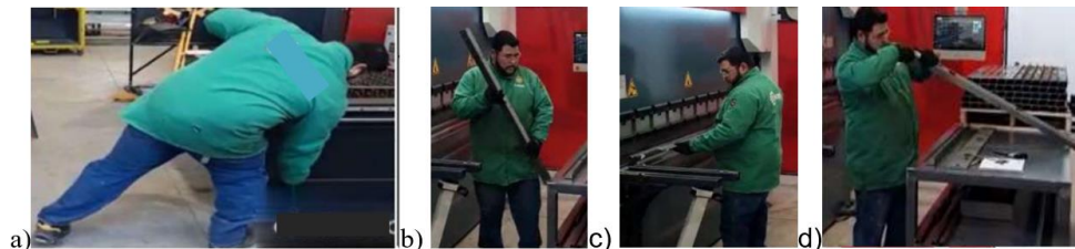
Figure 4. Sample: a) Material transportation, b) Material handling, c) Bending process and d) inspection
