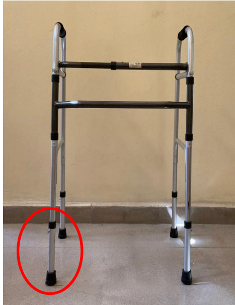
Figure 1. Folding walker with four legs and a one button release in each leg, highlighted with a red circle. See Figure 3.
