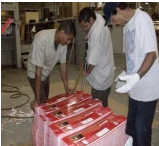
Figure 1.1 Preforming of boxes using the pneumatic roto- hammer
