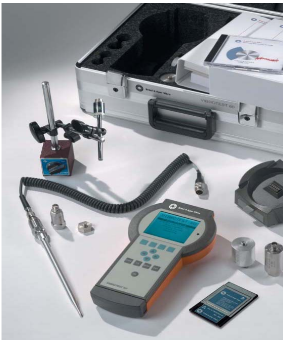
Figure 2.1 Vibrations Analyzer Utilized in the study
