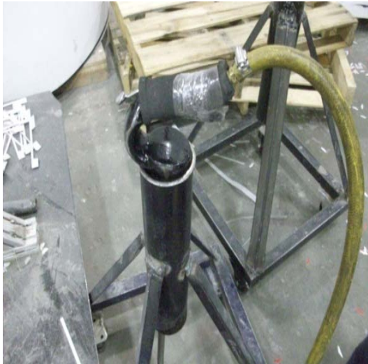
Figure 3.2 Insulation of tool handle
