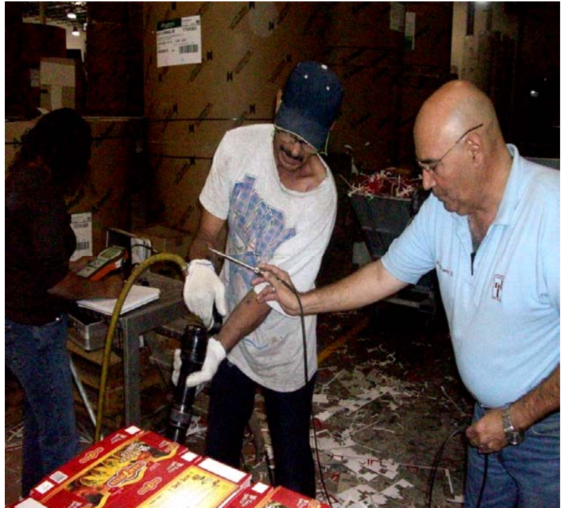
Figure 2.2 Vibrations readings taken at Stripping workstation.
