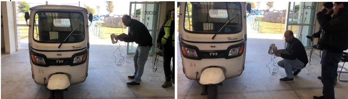
Figure 3. (Left) Scanning of the side section of the moto taxi 1. (Right) Scanning of the side section of the moto taxi 2.
