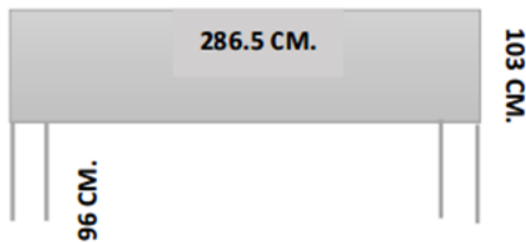
Figure 4 Current measurements of stainless steel tables.
