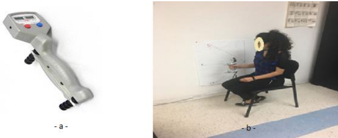
Figure 1. Devices used in the measurement of grip force. a) MicroFET® handgrip dynamometer. b) Cardboard.
