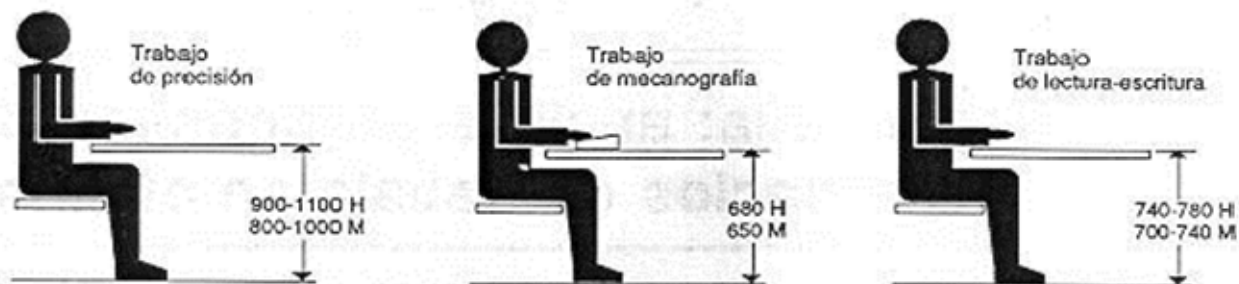
Fig. 1: Height of the level of work for sitting jobs (dimensions in mm) optimal scope zones of the working area
