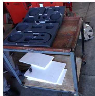
Figure 10. Work table with wheels for their management, compliance with measures for the convenience of the operator, without unnecessary movements.
