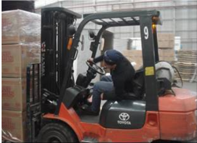
Figure 5. Visibility problem on the forklift.
