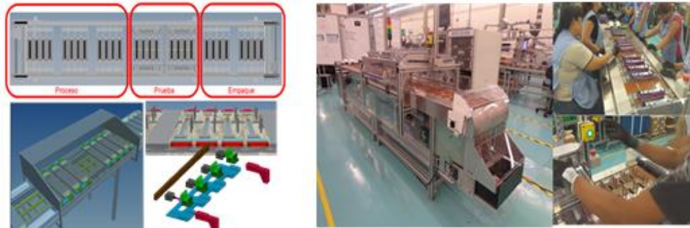
Figure 2. Semiautomatic Ergonomic System
