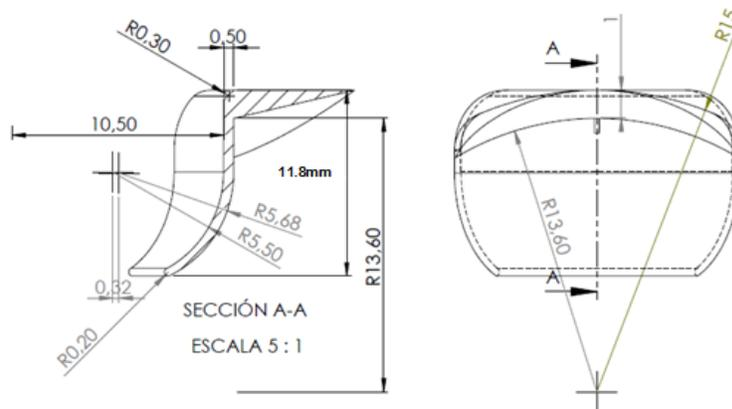
Fig. 13 Nail design, with an angle view and depth (11.8mm).
