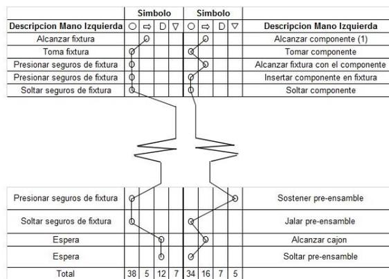
Figure 6. Bimanual diagram of the redesigned pre-assembly workstation.
