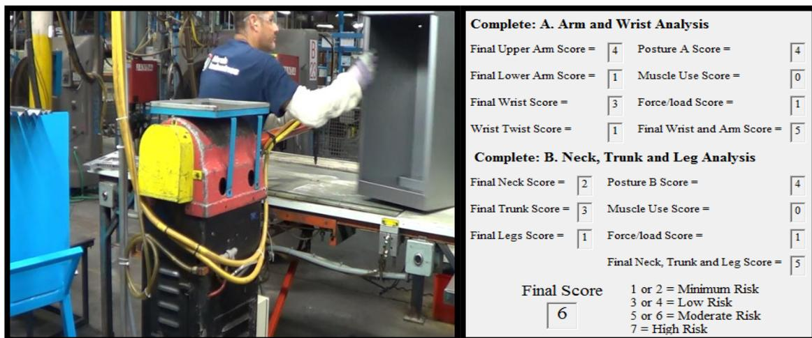
Fig. # 4. Operation: withdraw gauge, moderate risk.
