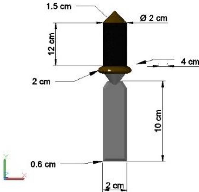
Figure 1. Guard and wood chisel design in AutoCaD (with measures).
