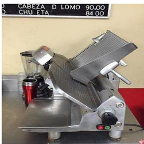
Figure 6. Slicing machine.
