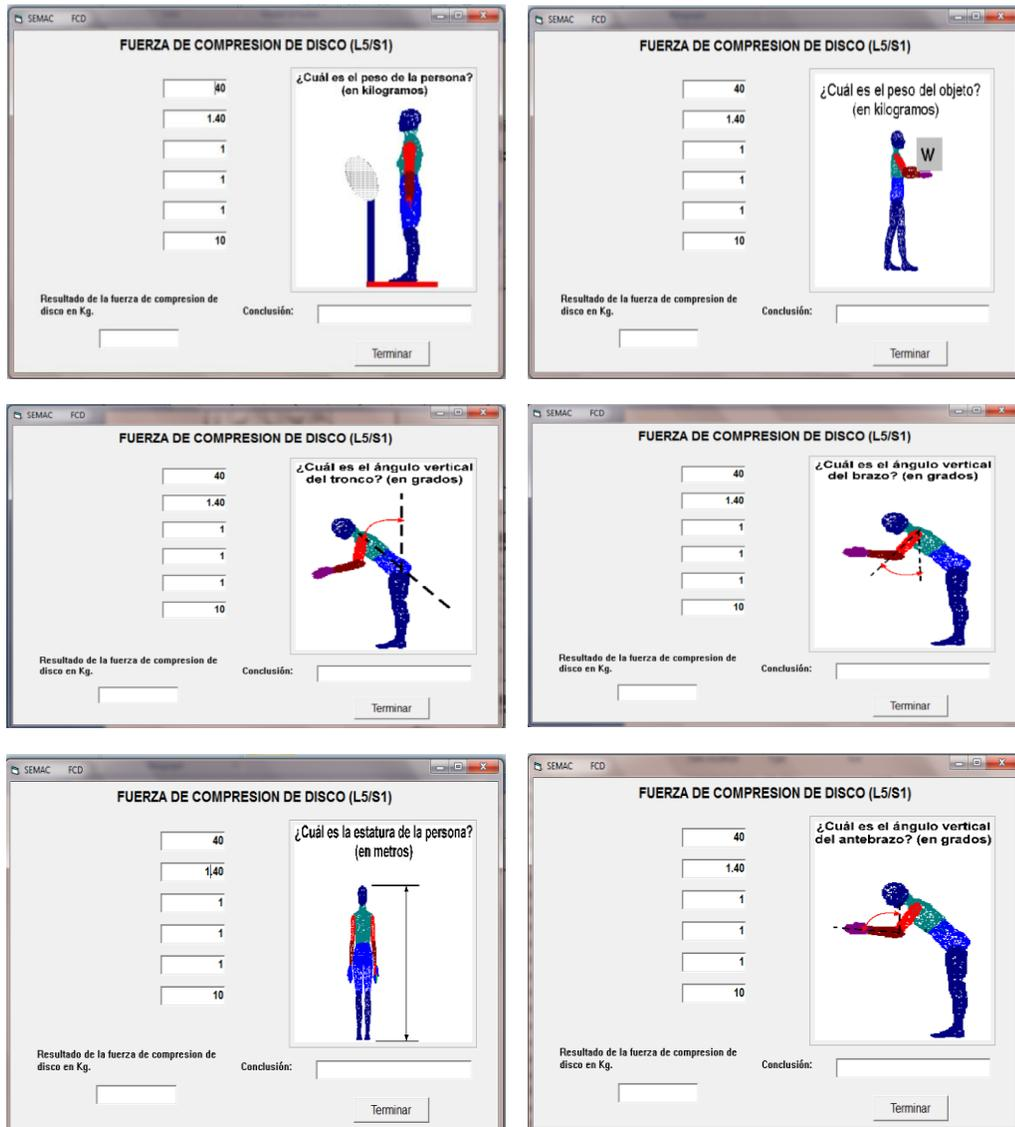
Fig. # 8. DCF Method Simulator
