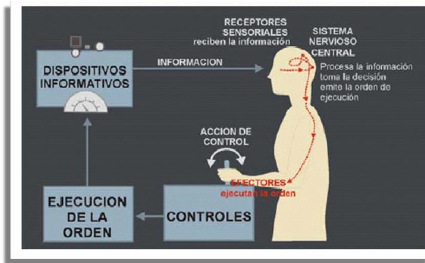
Fig. 2 Interrelations between the man-machine system.
