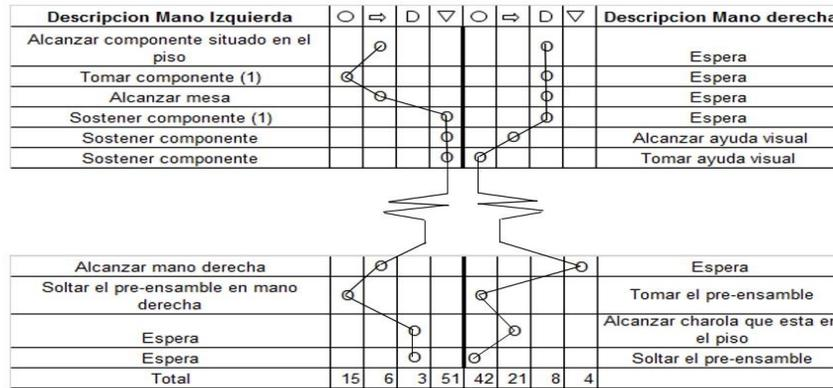
Figure 3. Bimanual diagram of the harness sub-assembly operation before the application of biomechanical principles and ergonomic guidelines.
