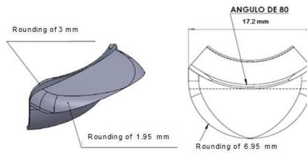
Fig. 12. Nail design, with top view and front view.
