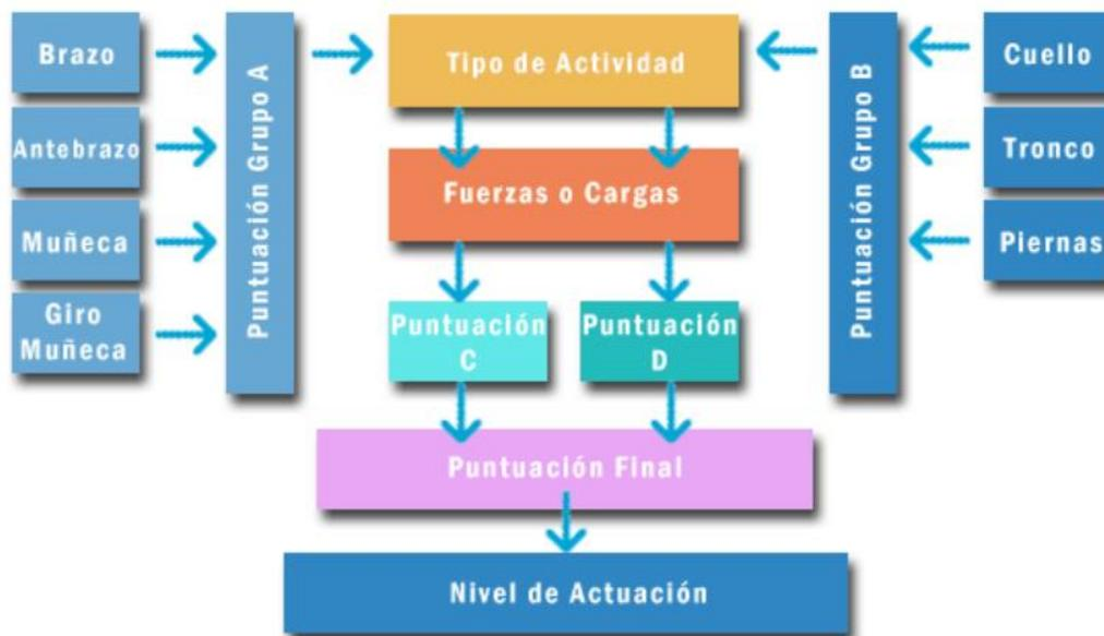
Figure 4. RULA Score Schema, source <https://www.ergonautas.upv.es/>
