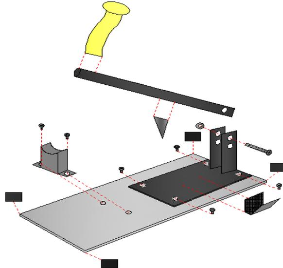
Figure 6. Drawing in press explosion to open clams.
