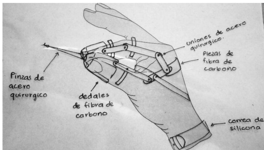
Fig. 2.0 Sketch guide for the design of the prototype of precision forceps. Shirley Navarro.
