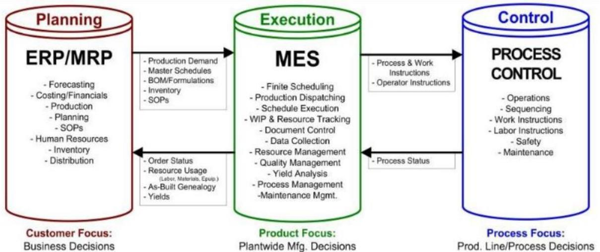
Figure 1. Relationship of an MES System in a Productive Process
