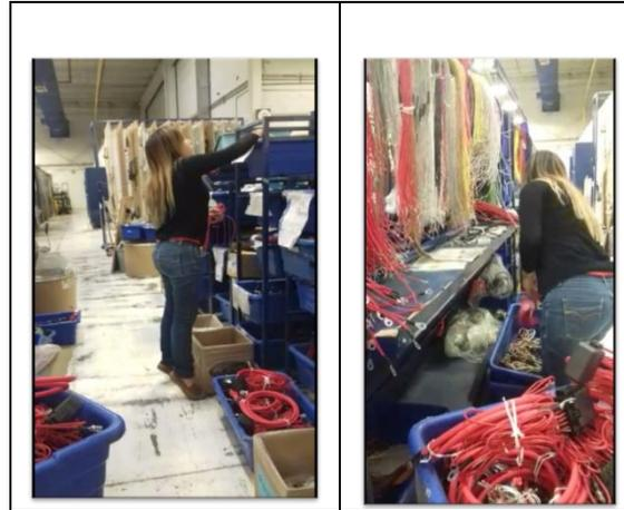
Figure 1. Harness pre-assembly station.
