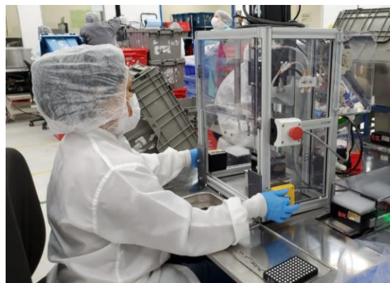
Figure 14. New protective cover in pressing station. Source. Own photography.
