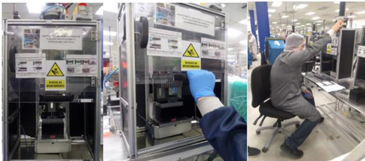
Figure 5. Pneumatic press with manual protective cover Source. Own photography.
