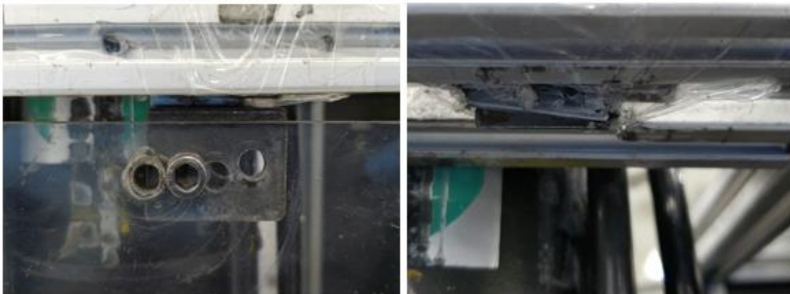
Figure 7. Magnet in charge of holding the door. Source. Own photography.
